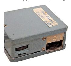
The receiver was controlled by a second three-position switch located at the other side of the control unit. In the centre position the receiver was switched off . The other two settings were: *EmR* (Empfang mit Rauschsperre - reception with squelch on), and *EoR* (Empfang ohne Rauschsperre - reception with squelch off). The volume control thumb wheel was on the left.
