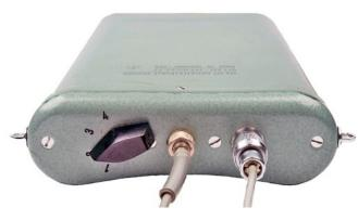
Top panel of the main unit, showing channel selector, microphone/speaker connection and aerial socket.
