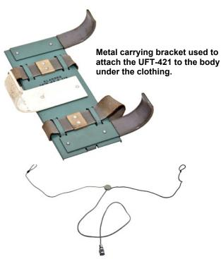
Two different types of aerials were issued with the UFT-421: a rod antenna and a wire antenna (shown above). The latter was an open dipole which could easily be hidden under the operator's clothing.
