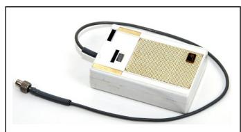
The loudspeaker/microphone of the UFT-421 was disguised as a commercial 'Mikki' medium wave transistor broadcast radio, using only the enclosure. These radios were commonly used in the GDR at the time and would not attract much attention to the public. It allowed the operator to hang around, pretending to be listening to a broadcast transmission, whilst in reality receiving instructions or passing status information.
